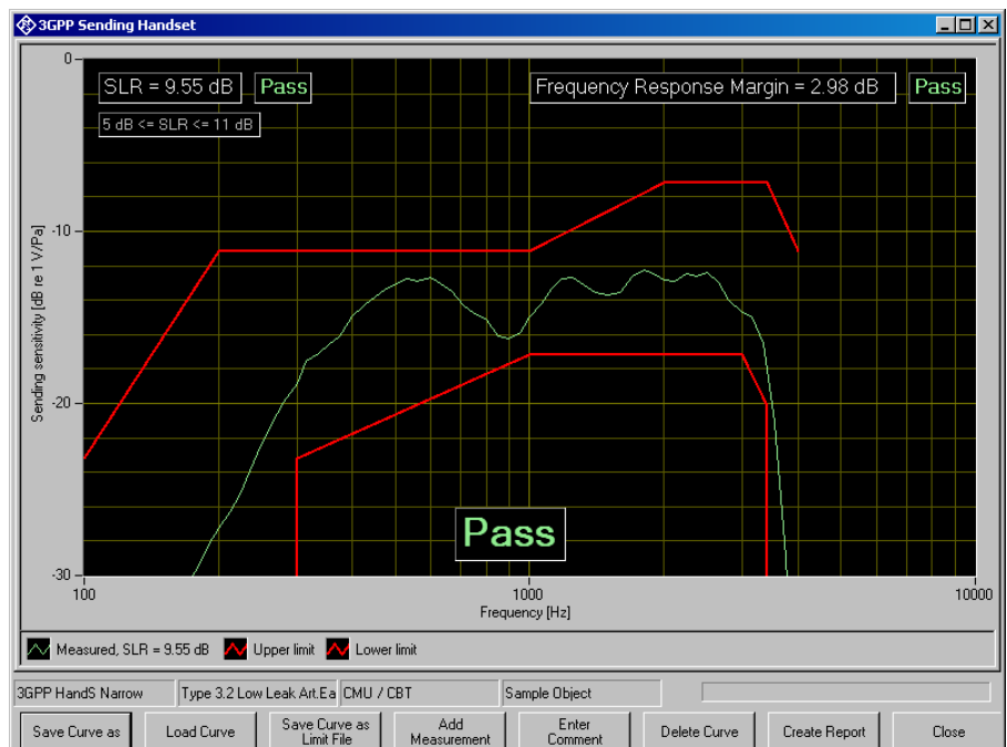
Fig. 37 Sending frequency response with SLR value displayed
