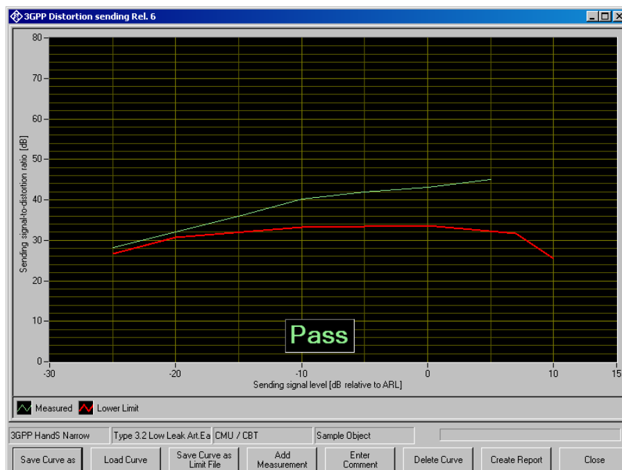
Fig. 46 Sending distortion measurement
