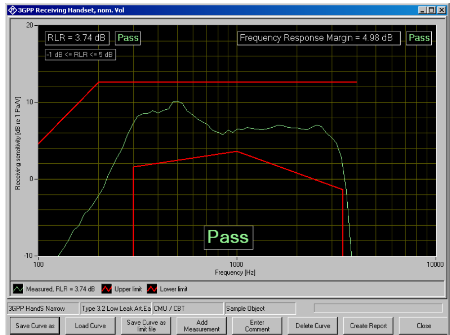
Fig. 38 Receiving frequency response with RLR value displayed
